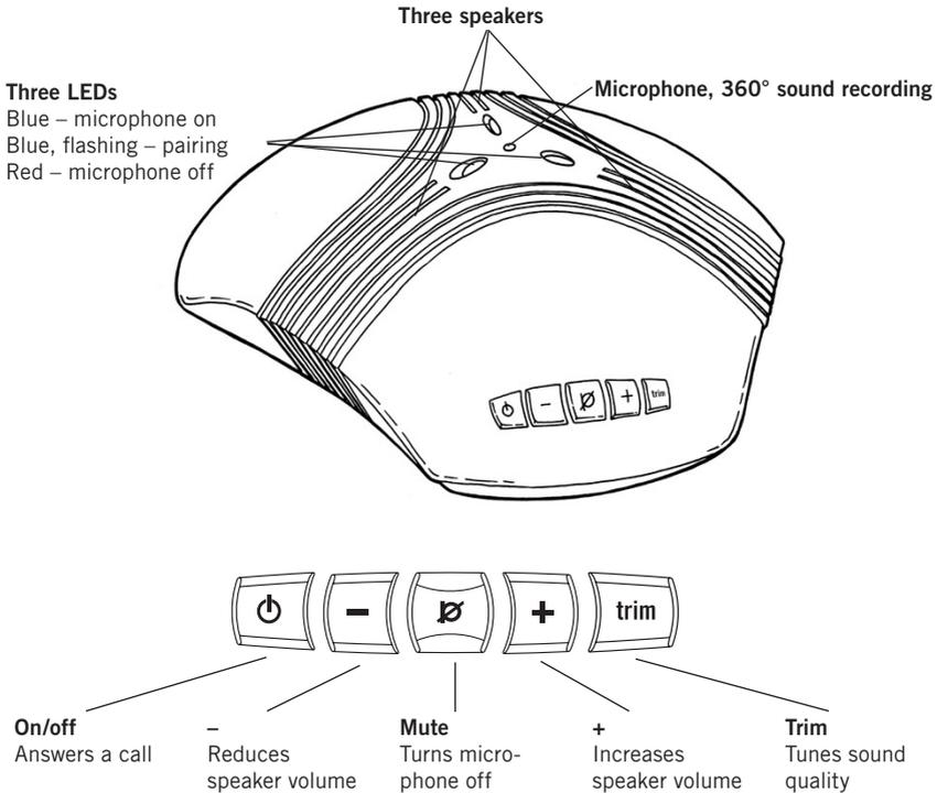
Konftel 60W is a conference unit for connecting to existing fixed system telephones, DECT telephones, mobile phones or computers, with a cable or wireless connection via Bluetooth. Konftel 60W has an omnidirectional, highly-sensitive microphone and three speakers which, together with Konftel's OmniSound® provide optimal sound quality and maximum reduction of room echo, even when the person speaking is standing at a slight distance from the unit.
