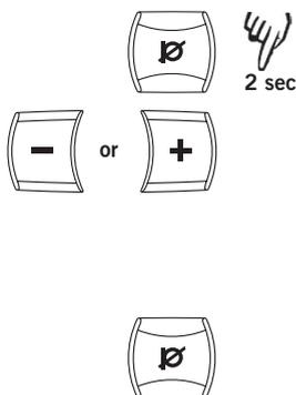
⇒ Press and hold the **mute** button for 2 seconds until the LEDs start to flash and you hear a tone.
