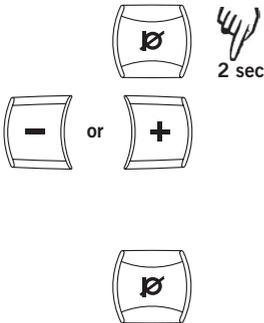
⇒ Press and hold the **mute** button for 2 seconds until the LEDs start to flash and you hear a tone.
